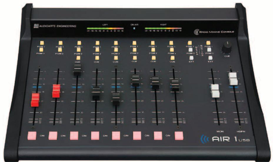
But the Audioarts engineers didn't take anything away from the design when they shrank it in the wash. The Air-1USB has two mic inputs, six line inputs and one USB Type B socket, speaker muting, selectable levels on inputs — really all of the things you see in competitors' consoles; *except* this mixer has two audio busses, a PGM 1 and PGM 2 line ("Audition" to you old-timers), just like the big boys have.
